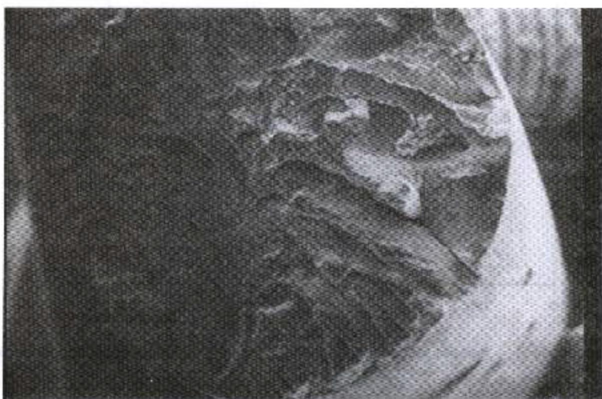
Fig.3: Typical fracture surface of the as received 5 mm diameter wires (AISI 1074 and 50B60) fractured under the rising load showing radial shear and longitudinal facets Mag. x 20.
